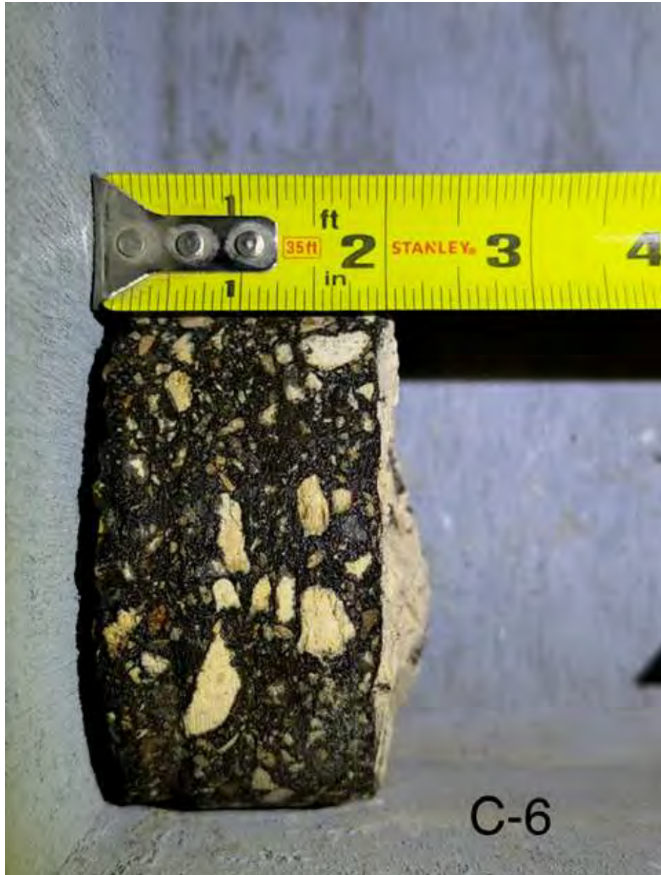
Photograph 6: Pavement Core C-6.
