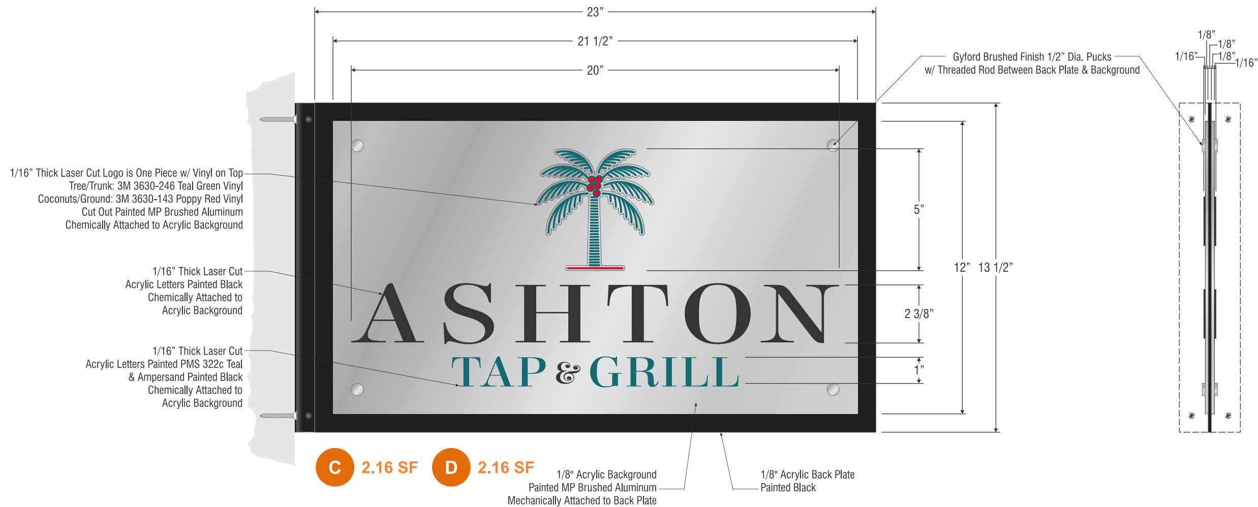
2 DOUBLE SIDED NON-ILLUM. WALL PLAQUE Scale: 3" = 1'-0"
